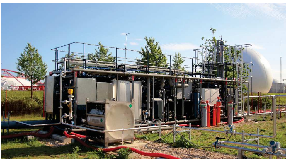
Figure 11 Cryogenic biogas upgrading and liquefaction, pilot plant from Cryo Pur, Valenton, France
